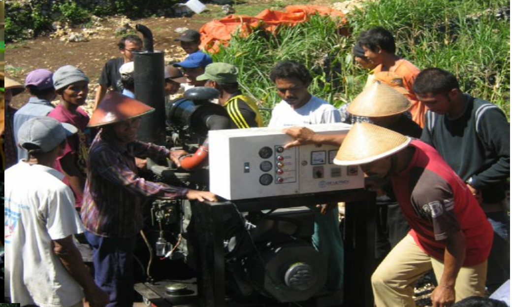
Electrical generator with 55kVA using biofuel
